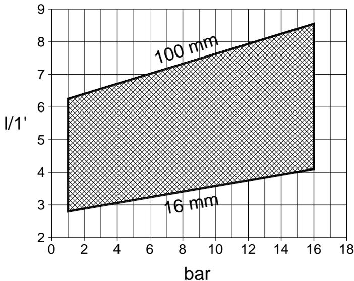
Tab. 3 - **REQUIRED LIQUID FLOW TO FLUSH MECHANICAL SEALS FROM OUTSIDE SOURCE**
